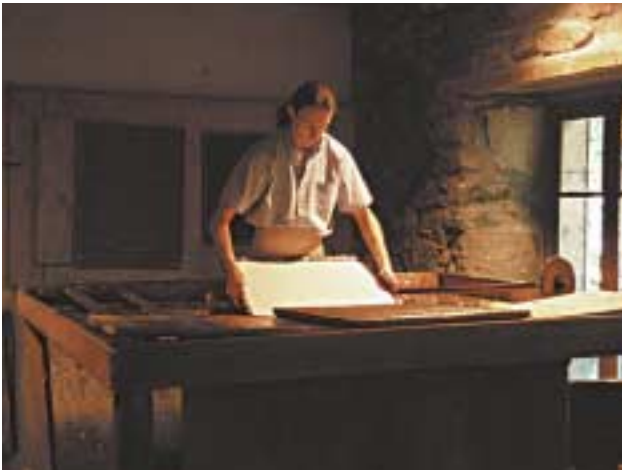
MAKING PAPER FROM CLOTH, MOULIN DE PEN-MUR, BRITTANY
